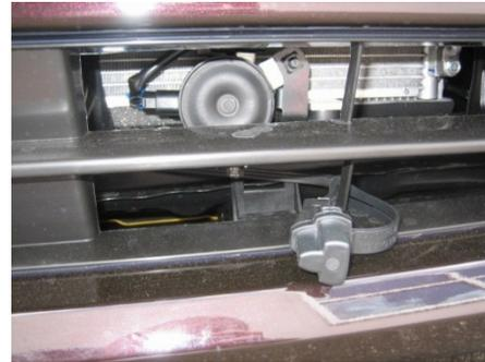
Using the male plug protector strap, attach the male plug to the grill-work in the lower air intake area.
