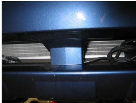
Route block heater harness in front of the A/C condenser and behind the vertical support for the lower air intake opening.
