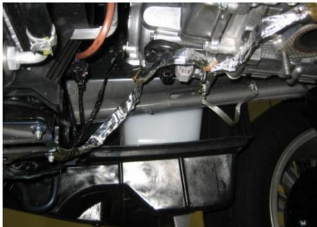
Plug harness into heater element. Orient orange connector towards the front by twisting the orange connector inside the heater. Inside of heater can be rotated relative to the outer body.
