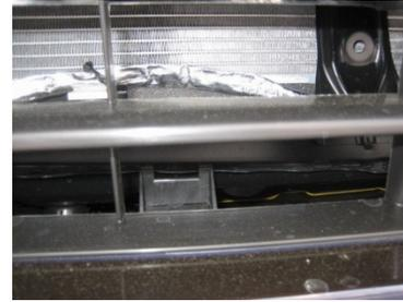
Route harness around the right side of the radiator and condenser towards the front of the car. Using a black wire tie included with the kit, attach the block heater harness to the A/C condenser bracket as shown.
