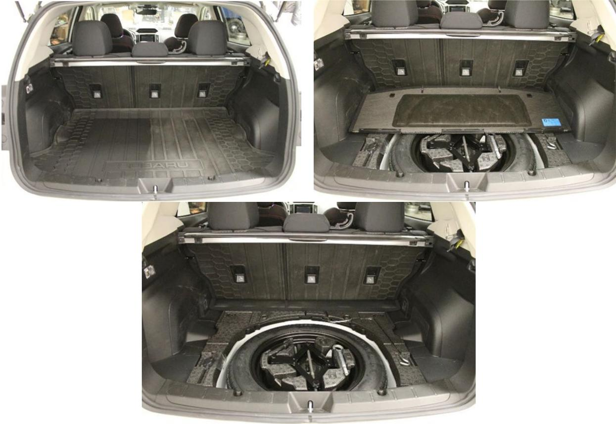
22. Remove the 4 clips holding the foam support liners, then remove the foam
