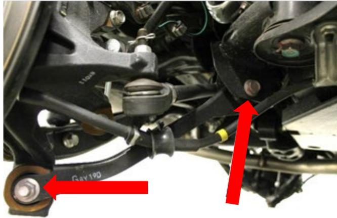
27. Loosen but do not remove the rear lower control arm bolt at the subframe (17mm socket).
