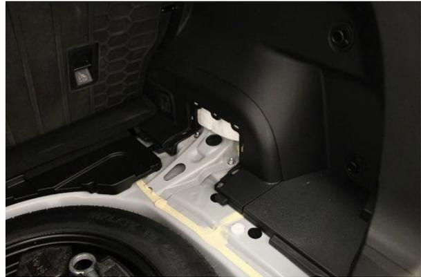
24. Remove the strut nuts and set aside (14mm Socket)
