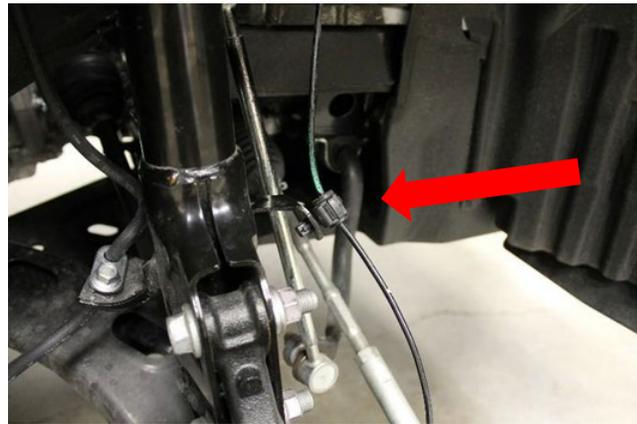
19. Install the front wheel and lower the vehicle to the ground. Torque the lug nuts to the wheel manufacturers specs. Jounce the front end to settle the suspension. Repeat process for opposite side of vehicle
