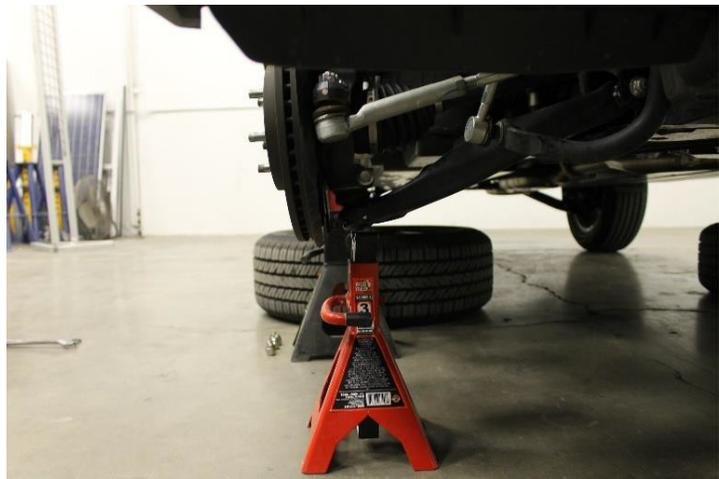
2. Remove the front sway bar end link at the strut body (17mm socket). This step should be completed on both sides to ease in installation at later steps.
