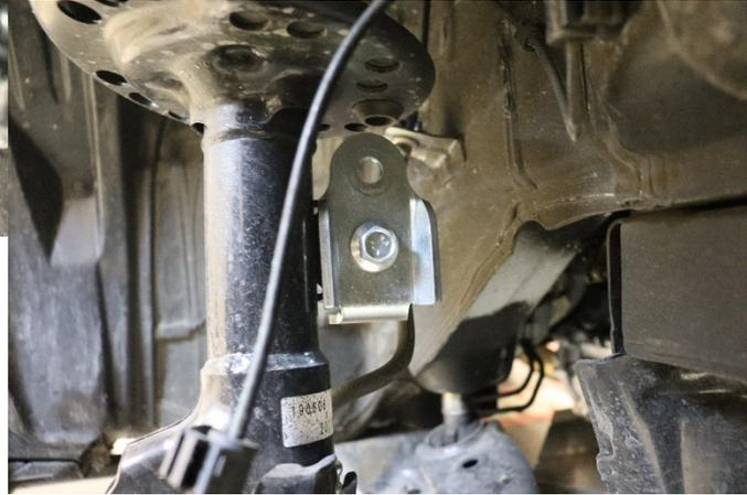
16. Install the 1/4" thick spacer washer onto the end link.
