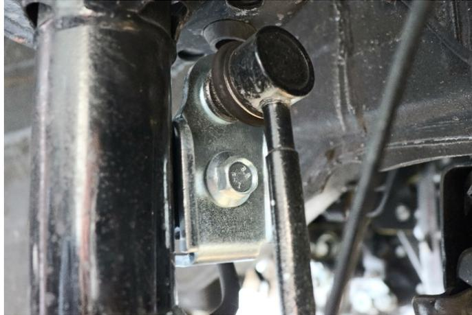
18. Install / Clip factory ABS wire harness onto strut
