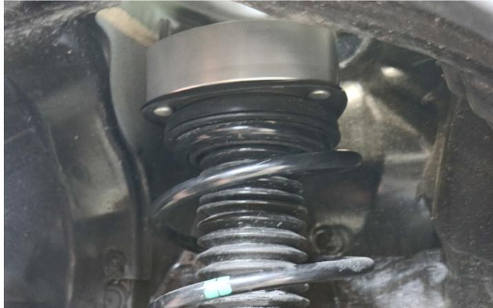
11. Align the three upper strut stud extension threads to the holes on the vehicle and fasten utilizing the factory flange nuts. When installed correctly, the Crawford Performance logo will be legible through the strut tower when facing the engine compartment. (Driver side shown)
