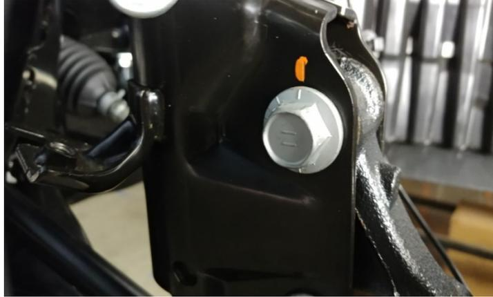
14. Install the brake line bracket to the strut body (12mm socket). Rotate the brake line bracket as shown. Originally the brake line was bolt- ed from the bottom upwards to the strut, now it will be mounted to the top of the strut body using the factory hardware.
