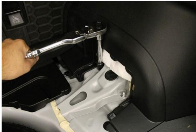
25. Loosen but do not remove the upper control arm bolts (17mm socket).
