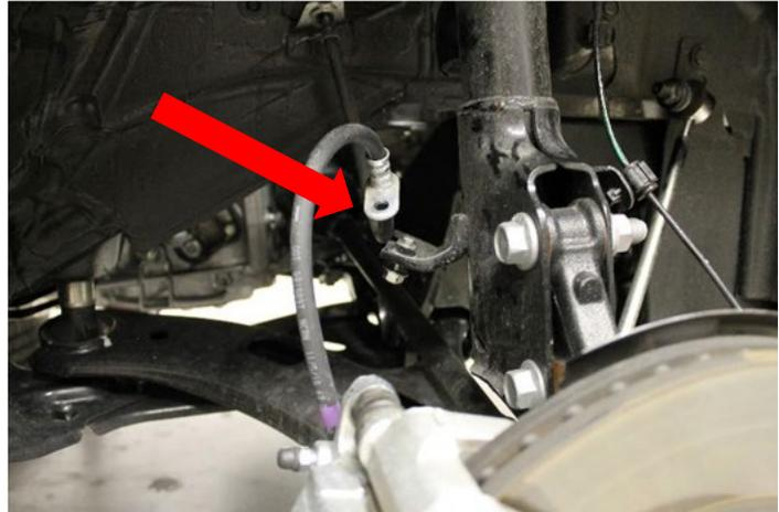
4. Remove the ABS harness clip at the strut body (flathead screwdriver). Let hang out of the way.
