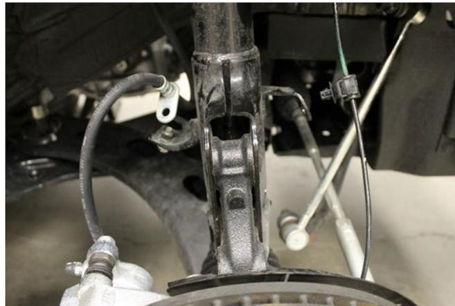
7. Remove the upper strut hardware (14mm socket). Make sure to hold the strut assembly from falling out of the vehicle. A helper is recommended for removal.
