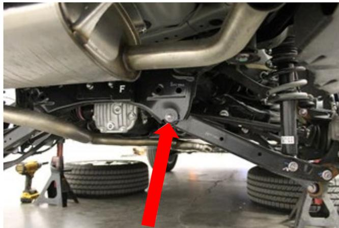
28. Remove both the factory lower rearward control arm bolt at the knuckle and the factory lower strut bolt (17mm socket), then lower the control arm and remove the factory strut assembly from the vehicle
