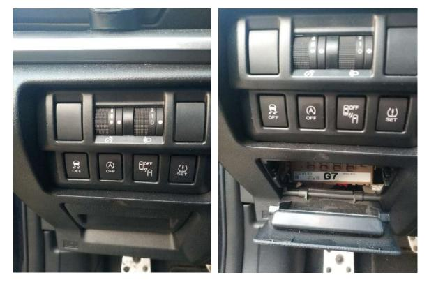
open the fuse box cover, and pushing inside the button block, extract it
