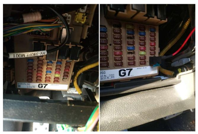
the power cable is connected to a free fuse socket, usually bottom right
