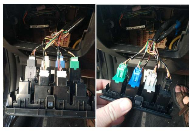
on connector has a key to connect (small projections on the left and right) you may need to remove with a sharp knife (it will not prevent from returning everything to its original state, if you want it)
