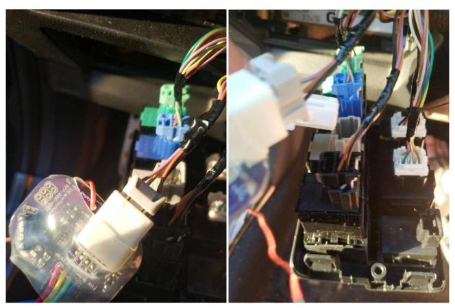
insert the car male connector into the female connector on the board
