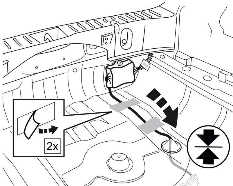
USING FOAM TAPE SECURE BLACK BOX, ENSURING IT DOES NOT INTERFERE WITH THE THRESHOLD.
