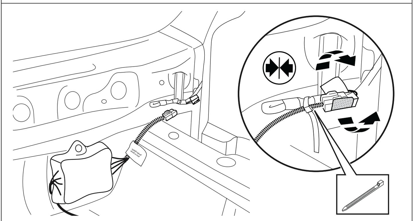
ROUTE 4 PIN FLAT CONNECTOR & HARNESS THROUGH EXPOSED HOLE, PAST GROMMET. PULL GROMMET BACK TO SEAT.
